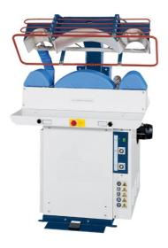
**Air operated press**for the finish of collars and cuffs of any type of shirts with stainless steel head.
