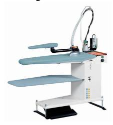
Vacuum ironing table. Manual heigth adjustment from 930 mm. to 750 mm. Very powerful vacuum with built-in vacuum unit operated by pedal. Manual vacuum deflection to the table or to the arm. Electrically heated board controlled by
