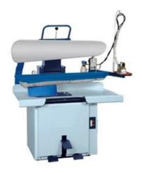
**Universal ironing Press**with stainless steel polished head ,steam heated but not steaming and padded buck with live steam and vacuum. The movement of the upper head is opearated by a pressure pedal, producing excellent results whilst being very easy to use and maintain . Available either for connection to external steam and vacuum supplies or self-contained. The built-in boiler can be powered to be connected to a second machine .
