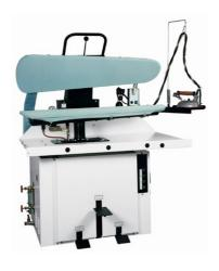
**Universal ironing Press**with padded buck and head. The movement of the upper head is opearated by a pressure pedal, producing excellent results whilst being very easy to use and maintain. Buck and head are both steaming and buck is also vacuum.
