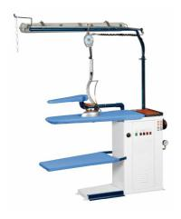
Electrically heated and vacuum table, utilityshape. It is supplied as standard with steam iron, vacuum unit and built-in electric automatic boiler able to operate an additional second iron on another table next to the FVC. It can be supplied by request with arm + sleeve's shape for spotting or finishing, steam or steam/air gun, cold spotting gun, water spray gun.
